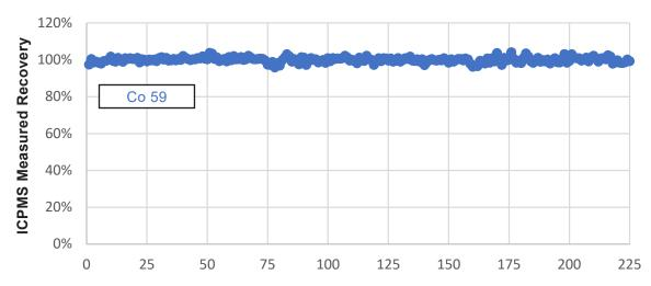
Automated internal standard (IS) addition to 225 sample filtrates using **TRAX**Station with LuerProbe. Each 10 mL filtrate was spiked with 0.1 mL of 100 ppb Cobalt (Co) IS stock solution. Cobalt was measured by ICPMS at m/z 59 with an average recovery of 100.0% and RSD of 1.3%, confirming the reproducibility and precision of the system for automated internal standard addition.
