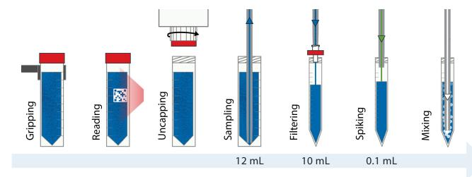
TRAXStation automatically and completely prepares samples for analysis. LuerProbe is used for sampling, filtering, spiking and mixing steps. Other probe options are available.
