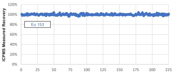
Automated acidification of 225 sample filtrates using **TRAX**Station with LuerProbe. Each 10 mL filtrate was spiked with 0.1 mL of 70%  $HNO_3$  containing 100 ppb Eu. Europium was added solely to generate a signal in the ICPMS mass spectrum (m/z 153), proportional to the amount of acid spike. The results demonstrated an average spike recovery of 99.9% with an RSD of 1.4%, confirming the reproducibility of the automated system.
